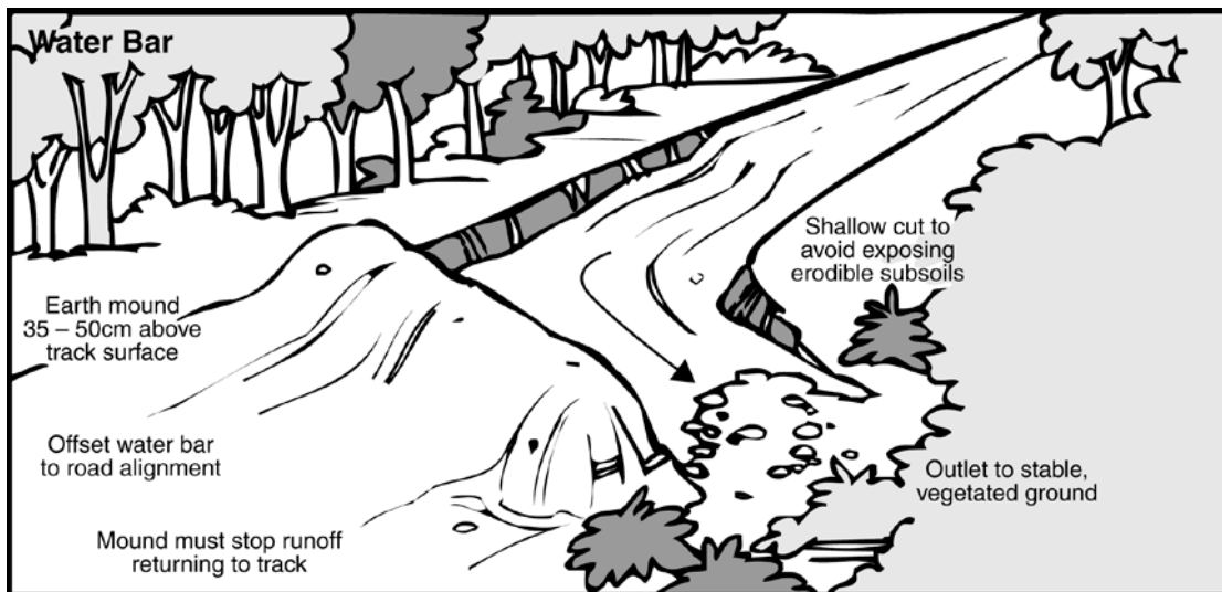
Diagram 9.3.5.4a – Water bar example
