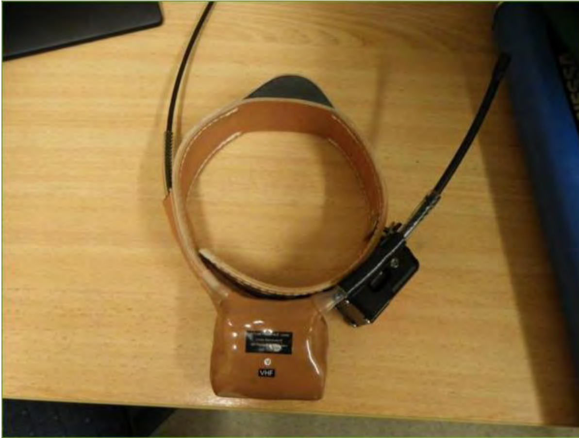
Figure 1. Example of the GPS collars fitted to dingoes. These units contained a GPS tracker, satellite transmitter, VHF transmitter, automatic drop-off mechanism and battery.
