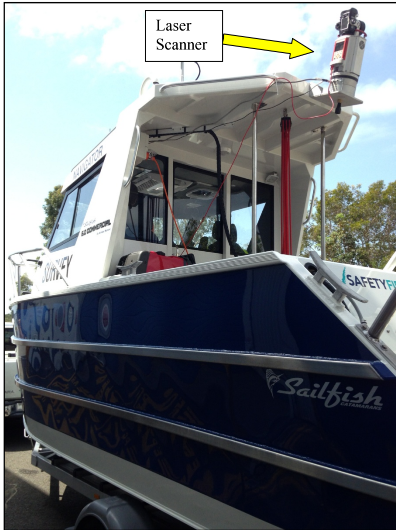
(Image No.4) Laser mount configuration on the ‘Navigator’
