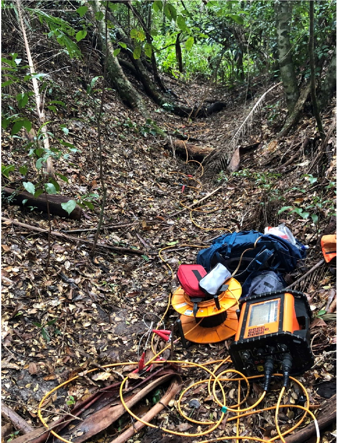
Figure 3-1 Typical survey setup of Terrameter LS, electrode pins and cables
