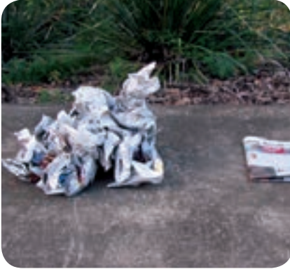
Photo 1a: The two samples above have the same fuel load (eighteen pages of newspaper) but a different fuel arrangement.
