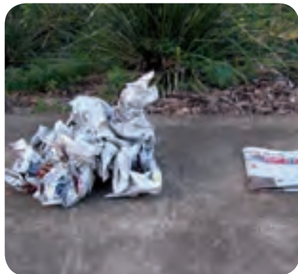
Photo 1a: The two samples above have the same fuel load (eighteen pages of newspaper) but a different fuel arrangement.
